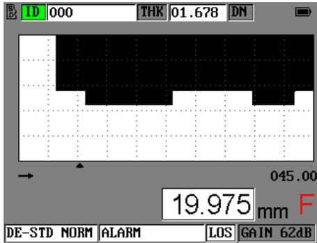
The TIME@2190 gage B-scan feature converts live thickness reading into cross-sectional images drawn on the display. This standard feature is very helpful in viewing the changes in thickness measurements over a distance. The B-scan is activated as soon as the transducer makes contact with the surface of the material.
