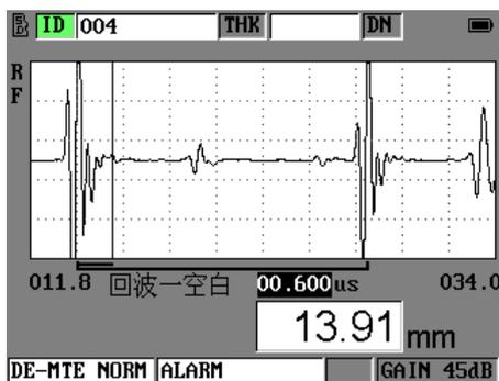
Measurement in manual E-E detection mode
