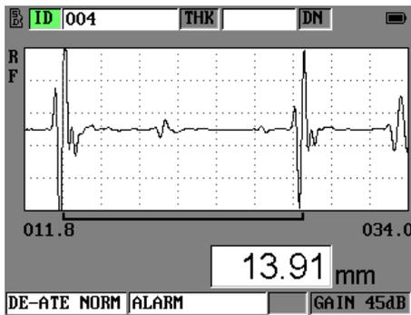
Measurement in automatic E-E detection mode
