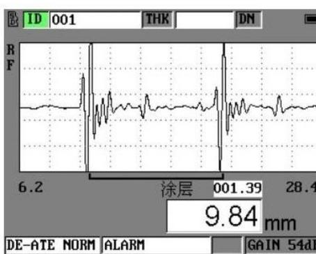
THRU-COAT mode with optional waveform
