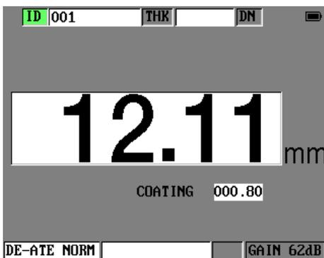
THRU-COAT mode showing the thickness of a coating and steel (waveform not activated)
